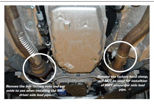
**STEP #1:** Remove the two nuts connecting the driver side lead pipe to the catalyst pipe. Set factory nuts aside they will be used for installation of the MRT driver side lead pipe.
